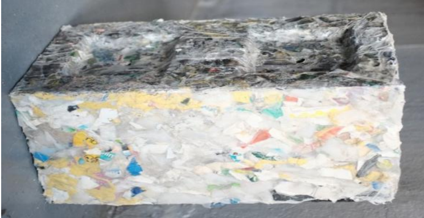
Building blocks made with plastics and rags
